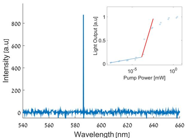
FIG. 5. Typical single mode lasing at  $586 \text{ nm}$  with a grating period of  $1.74 \mu\text{m}$  (corresponding to 9th Bragg order) with measured linewidth of  $0.22 \text{ nm}$ , limited by the spectrometer. Inset shows a typical pump light vs light output, laser threshold about  $10^{-4} \text{ mW}$ .
