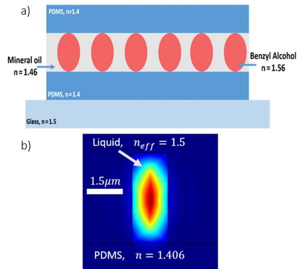
FIG. 4. (a) Schematic side view of the lasing device with refractive index of each component. Typical period is in the range of 1.3–5  $\mu\text{m}$ . Channel height is about 5  $\mu\text{m}$  and its width is about 2  $\mu\text{m}$ . Generally, the droplets are elliptical in shape. (b) The normalized electric field pattern of in-plane fundamental mode of the liquid waveguide with dimensions of 1.5  $\mu\text{m} \times 5 \mu\text{m}$ .
