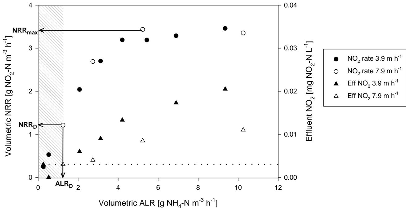
**Figure 5: Volumetric nitrite removal rate (left axis) and effluent nitrite concentration (right axis) as a function of volumetric ammonium loading rate. The shaded area shows the safe operating window for nitrite removal and the dotted line shows the regulatory limit for nitrite (0.003 mg NO<sub>2</sub>-N L<sup>-1</sup>). The NRR<sub>d</sub> shows the maximum NRR achieved to meet Danish drinking water guidelines.**
