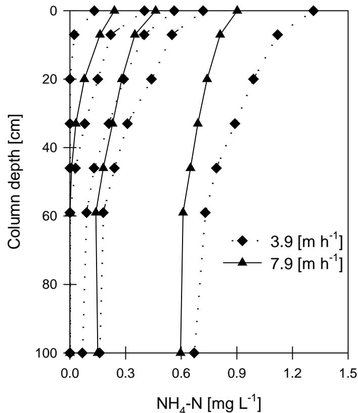
**Figure 6: Ammonium depth profiles at hydraulic loading rates of  $3.9$  and  $7.9 \text{ m h}^{-1}$ . The influent water is represented by a depth of  $0$  while the effluent is shown as a depth of  $100 \text{ cm}$ .**
