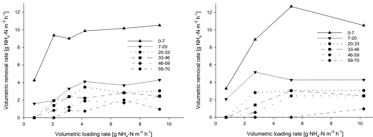
Figure 1A: Volumetric NH<sub>4</sub>-N removal rate of ammonium [g NH<sub>4</sub>-N m<sup>-3</sup> h<sup>-1</sup>] as a function of volumetric NH<sub>4</sub>-N loading rate [g NH<sub>4</sub>-N m<sup>-3</sup> h<sup>-1</sup>] at different depths in the filter for hydraulic loading rates of 3.9 m h<sup>-1</sup> (left) and 7.8 m h<sup>-1</sup> (right).
