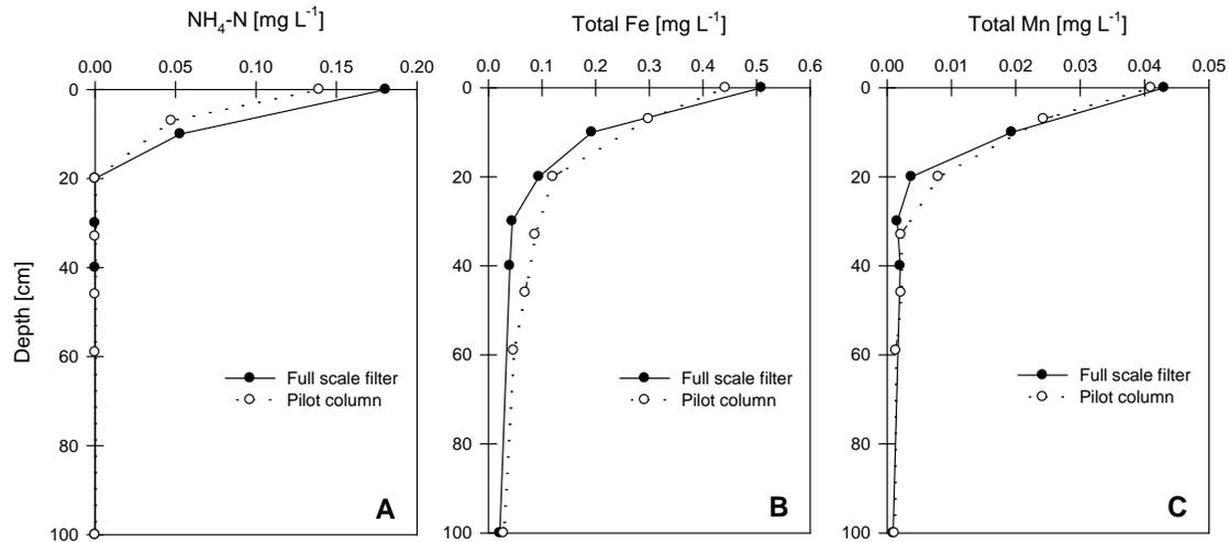
**Figure 3: NH<sub>4</sub>-N, total Mn, and total Fe depth profiles for Islevbro full-scale filter and the pilot column operating under reference conditions. All samples were collected on the same day, 4 months after the startup of the pilot column.**
