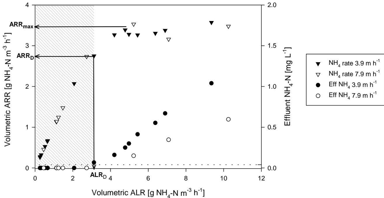
**Figure 4: Volumetric ammonium removal rate (left axis) and effluent ammonium concentration (right axis) as a function of volumetric ammonium loading rate. The shaded areas show the safe operating window for removing ammonium and the dotted line shows the regulatory limit for ammonium ( $0.04 \text{ mg NH}_4\text{-N L}^{-1}$ ).  $ALR_d$  and  $ARR_d$  show the maximum acceptable ammonium loading and removal rates for Danish drinking water guidelines.**
