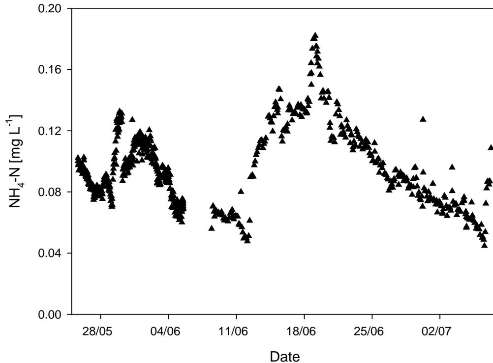
**Figure 1: Inlet ammonium concentrations for the feed water supplying both the full-scale filters and pilot column at Islevbro water works in the summer of 2012. Outlet ammonium concentrations were all below the quantifiable limit of  $0.02 \text{ mg NH}_4\text{-N L}^{-1}$ .**
