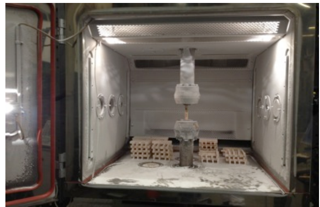
Figure 1: Climate chamber, shear test machine and test specimens
