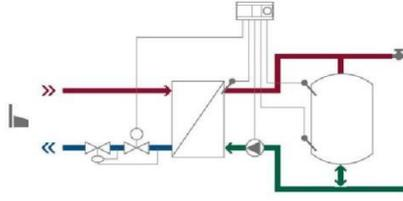
Figure 3.(b). DHW preparation with HEX + tank
