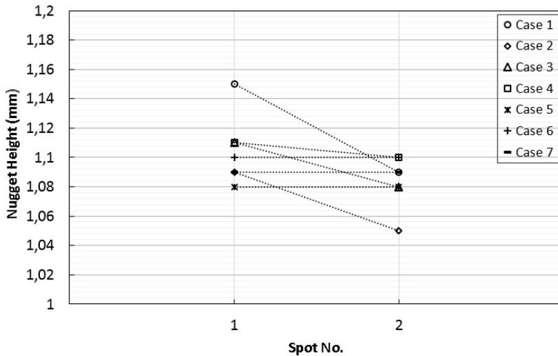
**Fig. 6** Comparison of 1<sup>st</sup> and 2<sup>nd</sup> Nugget Height Measured by Metallographic Examination.
