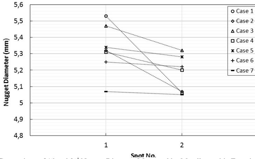
**Fig. 5** Comparison of 1<sup>st</sup> and 2<sup>nd</sup> Nugget Diameter Measured by Metallographic Examination.
