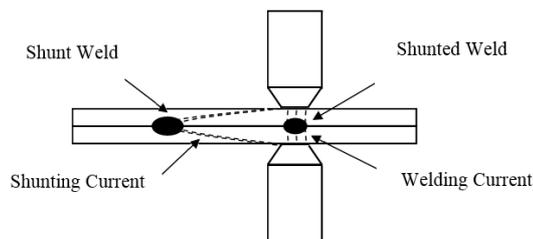
**Fig. 1** Schematic Representation of Shunting in Spot Welding.
