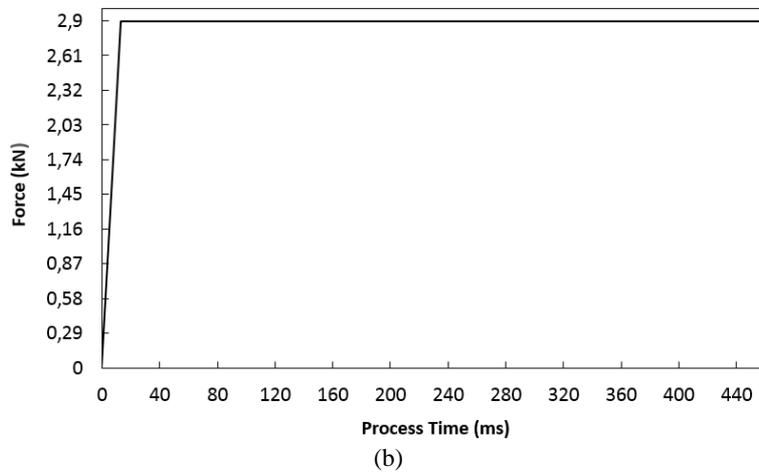
**Fig. 2** Optimal Welding Schedule Specifications (a) Welding Current, (b) Electrode Force.
