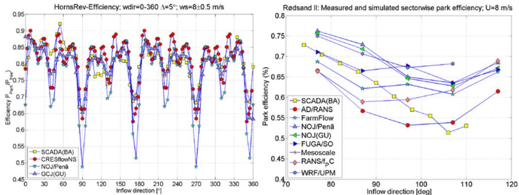
Fig. 1. Wind farm wake observed from SCADA data and wake models results at Horns Rev 1 for 360° and for Rødsand 2 for 41° in the eastern sector where SCADA data was available.
