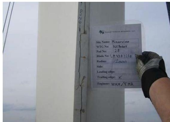
Figure 7 Fatigue failure in bondlines, longitudinal cracks in the trailing edge
