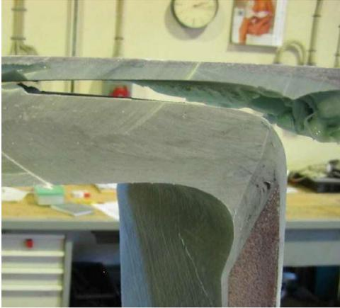
Figure 4 Delamination - faulty injection
