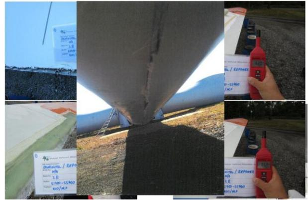
Figure 11 Transport damage
