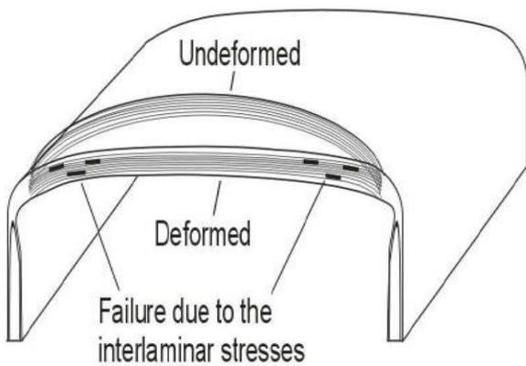
Figure 2 Interlaminar failure
