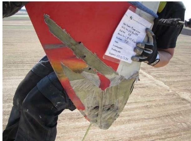
Figure 9 lightning damage
