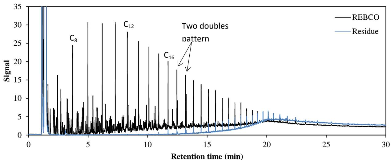
Figure 4. GC spectra of fresh REBCO and a REBCO residue. The two doubles pattern of heptadecane-pristane and octadecane-phytane as well as the peaks representing *n*-octane, dodecane and hexadecane are marked.
