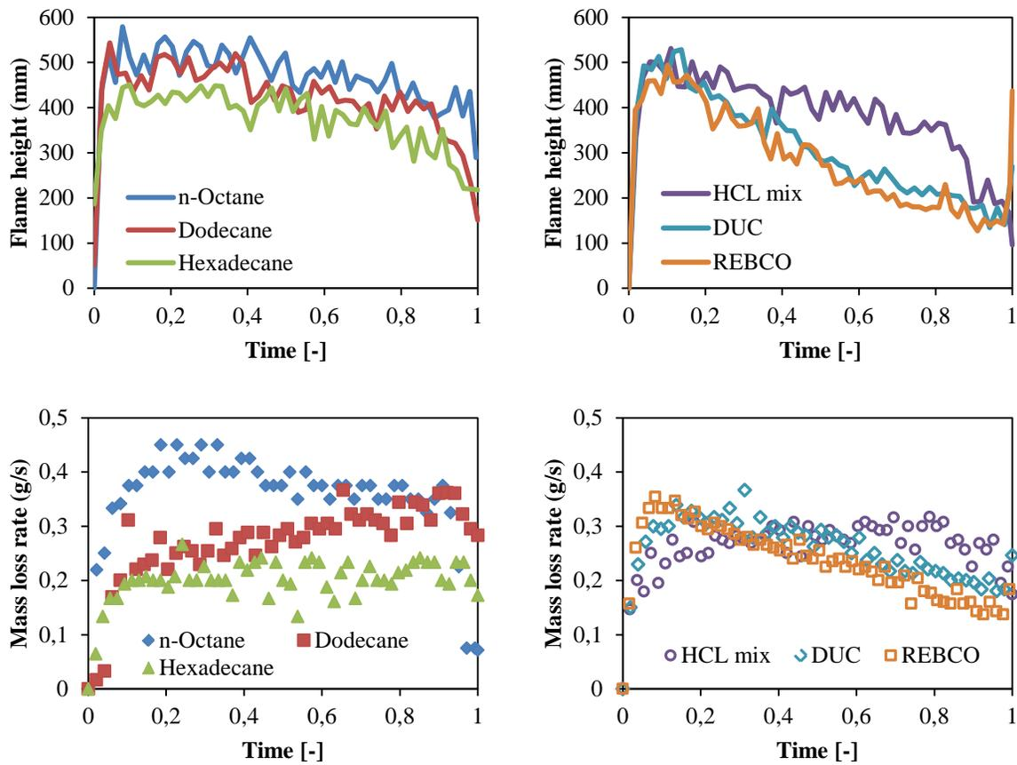
Figure 3. Flame height (top left) and mass loss rate (bottom left) as a function of time for *n*-octane, dodecane and hexadecane and flame height (top right) and mass loss rate (bottom right) for the HCL mixture, DUC and REBCO.
