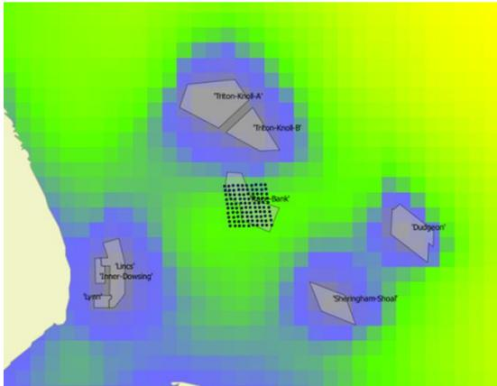
Figure 2: Wind resource with influence of neighboring wind farms in a wind farm cluster. Calculations with the WRF model.
