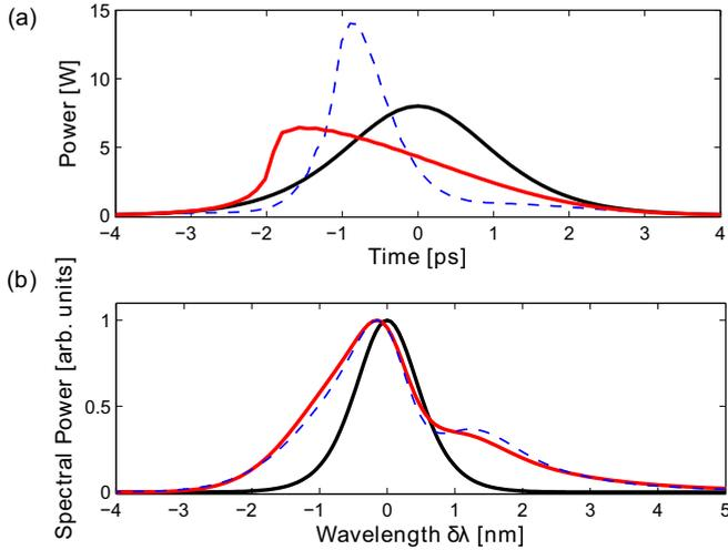
FIG. 2. (Color online) (a) Temporal and (b) spectral pulse properties of *anomalous* self-steepening in PhC waveguides. Notice the behavior is opposite to unstructured media exhibiting normal self-steepening. Traces are shown for propagation of  $200 \mu\text{m} \approx 2.5L_{\text{NL}}$ . Legend: Kerr and SS only (thick red), full Eq. (1) (dashed blue), and input pulse (black).
