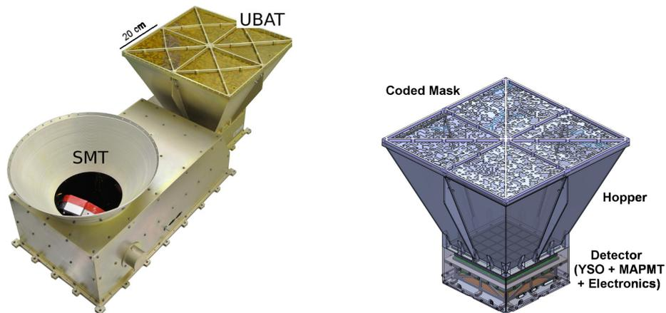
**Figure 1:** *Left:* A photo shows the assembled UFFO-p with its two scientific instruments: UBAT and SMT. *Right:* A schematic view of UBAT is drawn. It consists of a coded mask, hopper, detector and readout electronics.
