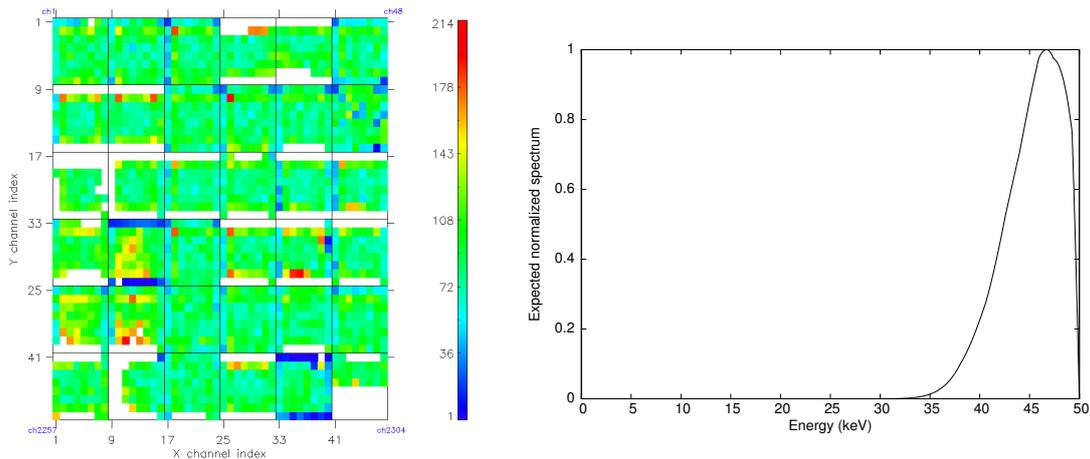
**Figure 2:** *Left:* The UBAT FM detector response to X-rays of energies  $\leq 50$  keV is shown. The color scale indicates the total number of counts in each pixel. White color means zero counts at noisy detector pixels, which have been disabled noisy. *Right:* The expected normalized spectrum given by the radiation produced by the X-ray tube illuminating the detector after attenuation in the air and in the Cu filter is displayed.
