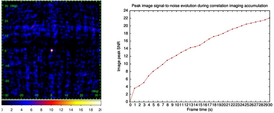
**Figure 3:** *Left:* Reconstructed X-ray image as an SNR map. Color scale corresponds to the SNR value. The X-ray tube was placed on axis with voltage 50 kV. The X-ray source is clearly visible in the middle of the FOV. *Right:* The image peak SNR evolution during the exposure time.
