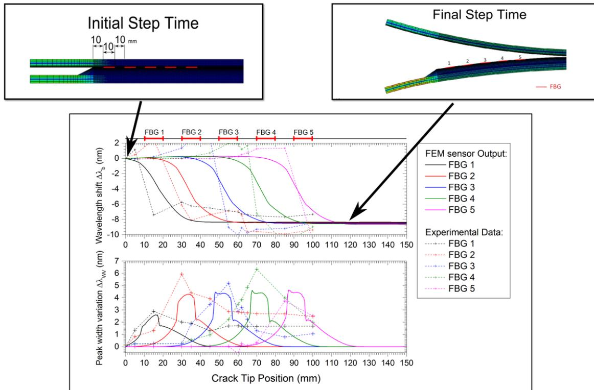
Figure 3: Model experimental validation: FBG Output prediction.
