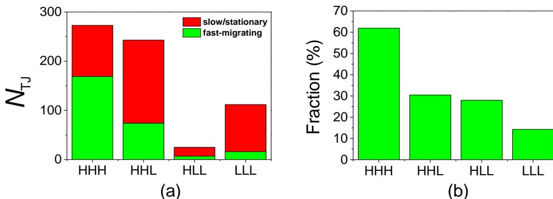
**Figure 4.** Populations of different TJs investigated in one region both in the deformed condition and after 10 min at 170 °C: (a) frequencies of TJs classified as either fast-migrating or slow/stationary; (b) fractions of fast-migrating junctions in each TJ group.
