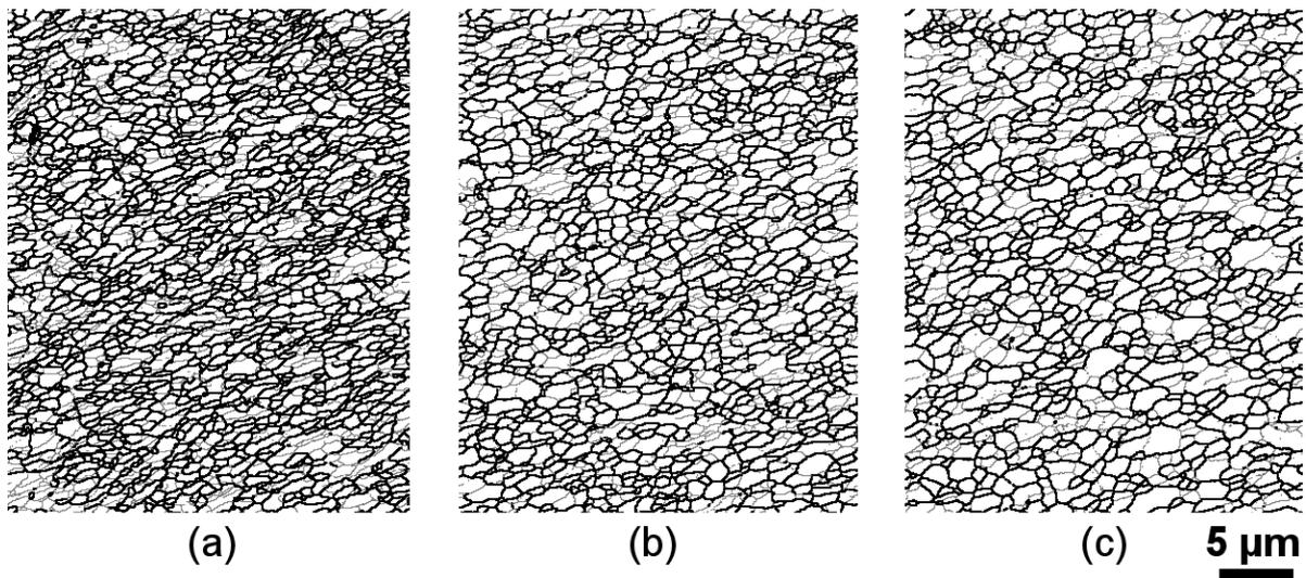
**Figure 1.** EBSD maps representing the microstructure of aluminum after ECAE (a) and subsequent annealing at  $170^\circ\text{C}$  for 10 minutes (b) and 2 h (c). Gray and black lines show LABs and HABs, respectively. The extrusion direction is parallel to the scale bar.
