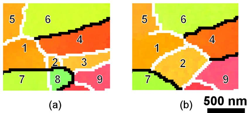
**Figure 5.** An example showing migrating LLL-type junctions (a) before and (b) after annealing at  $170^\circ\text{C}$  for 10 minutes. White and black lines show LABs and HABs, respectively. Numbers mark subgrains present in this area.
