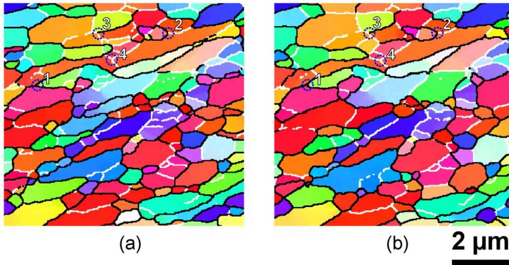
**Figure 3.** Changes in one region mapped using the EBSD technique in the deformed condition (a) and after annealing at 170 °C for 10 minutes (b). White and black lines show LABs and HABs, respectively. Examples of four different TJ types considered in this work are marked by blue circles and numbers: 1 – HHH, 2 – HHL, 3 – HLL and 4 – LLL. The extrusion direction is parallel to the scale bar.
