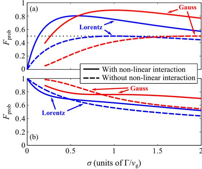
FIG. 4. (Color online) Degree of directional entanglement  $F_{\text{prob}}$  plotted for varying incoming pulse widths, shown for both Lorentzian and Gaussian input pulses (solid lines). The corresponding values obtained when neglecting two-photon-scattering terms are also shown (dashed lines). (a) Pulse and emitter are resonant,  $\Delta = 0$ . (b) Pulse and emitter detuned by  $\Delta = \Gamma/(2v_g)$ .
