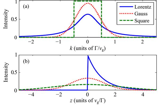
FIG. 2. (Color online) (a) Intensity spectra,  $|\xi(k)|^2$ , for the three single-photon wave packets in Eqs. (13)–(15), here plotted with  $\sigma = \Gamma/v_g$ . (b) Corresponding spatial pulse profiles,  $|\xi(z)|^2$ , with large values of  $z$  corresponding to the front part of the pulse, arriving first at the position of the emitter.
