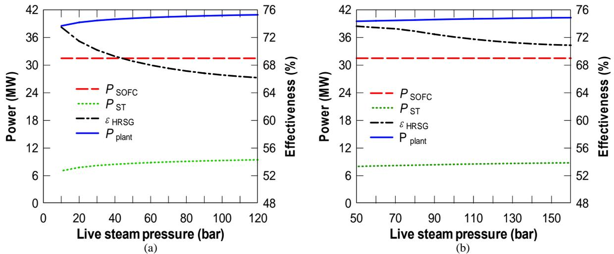
Fig. 6 Effect of live steam pressure on plants net power output and HRSG effectiveness: (a) Case C; (b) Case D.
