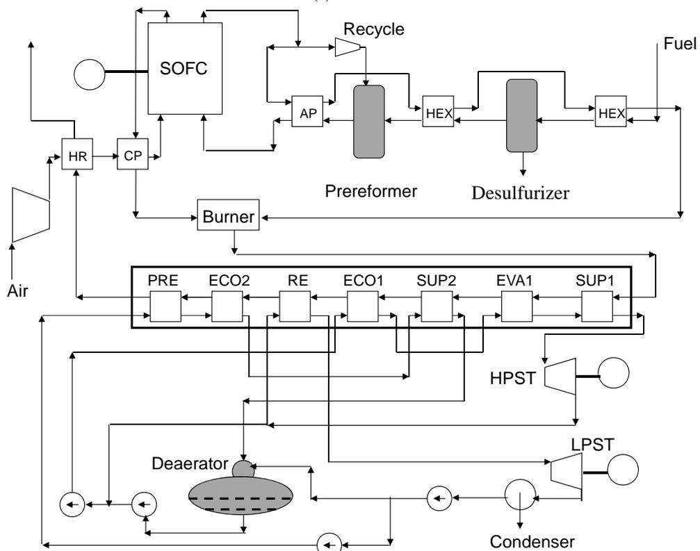
Fig. 2 Combined SOFC-ST plant with hybrid recuperator, (a) single pressure Rankine cycle and (b) dual pressure Rankine cycle.
