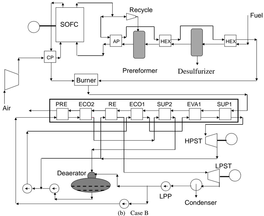
Fig. 1 Combined SOFC-ST cycle plant without hybrid recuperator, (a) single pressure Rankine cycle and (b) dual pressure Rankine cycle.
