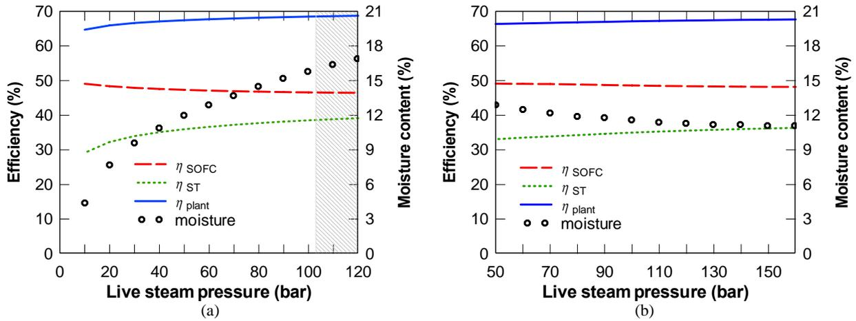
Fig. 4 Effect of live steam pressure on plants efficiencies and moisture content: (a) Case C; (b) Case D.
