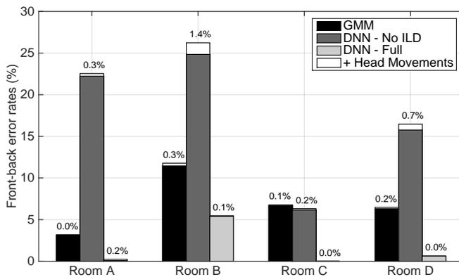
**Fig. 2.** Front-back error rates produced by different systems without head movements (shaded bars) and with head movements (white bars) in different room conditions. The error rate numbers for the white bars (with head movements) are displayed at the top of the bars. The task was single-speaker localisation.
