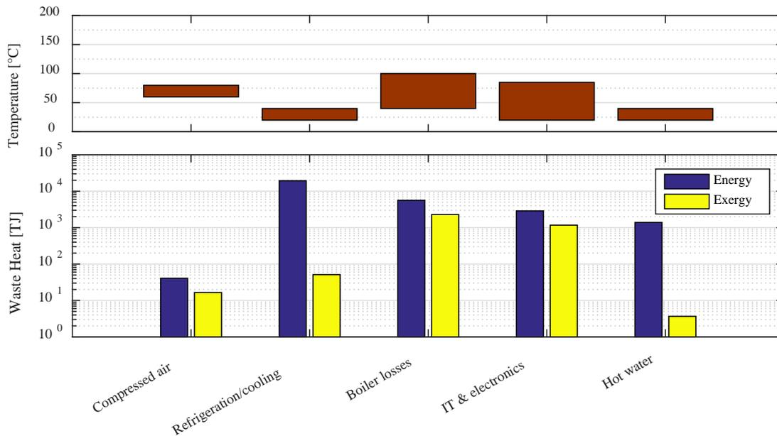
Fig. 3. Waste heat and temperature intervals for the different processes in the building sector.
