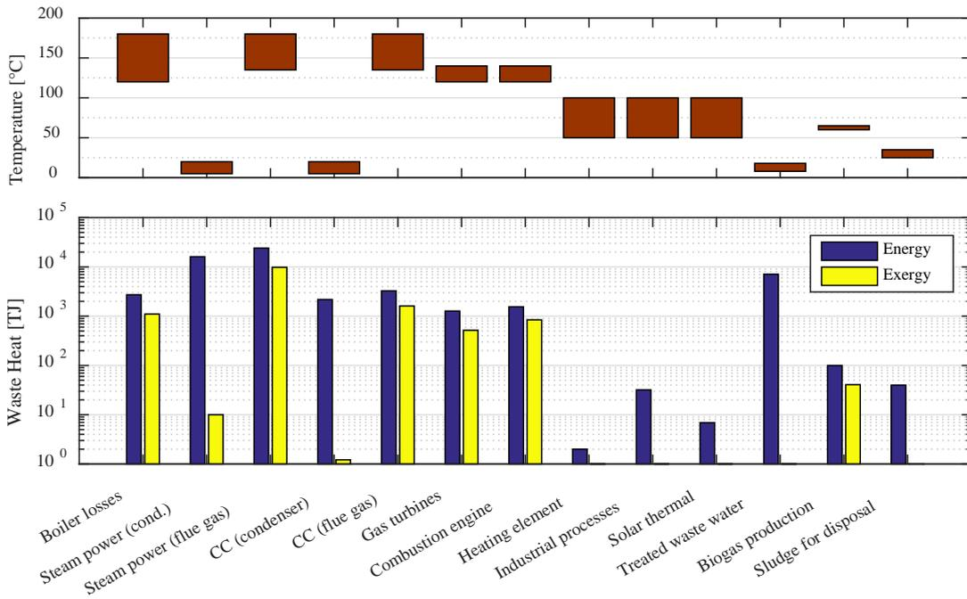
Fig. 4. Waste heat and temperature intervals for the different processes in the utility services.
