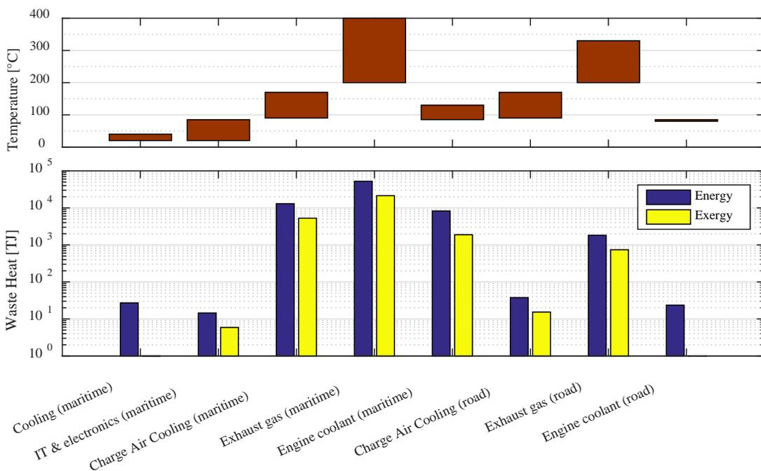
Fig. 5. Waste heat and temperature intervals for the different processes in the transport category.
