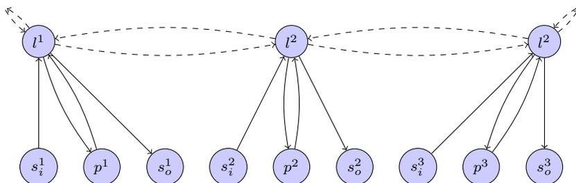
**Fig. 2** The structure for a single line at one frequency visiting multiple stations. Each station has three vertices; a source vertex  $s_i$ , a sink vertex  $s_o$ , and a platform vertex  $p$ . All passenger paths originate from some source vertex, and terminate at some other sink vertex, travelling on dashed line travel edges or switching lines using a platform vertex.
