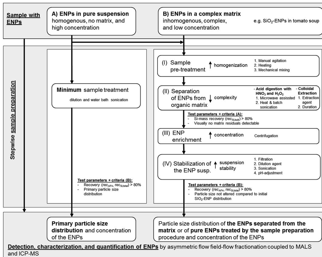
Fig. 1 Generic multi-step procedure for development of a sample preparation method to extract ENPs from a complex matrix. Specific details for the example separation of  $\text{SiO}_2$ -ENPs from tomato soup are given on the right side of the scheme (numbered sub-steps can be performed as stand-alone or in combination with other listed sub-steps).
