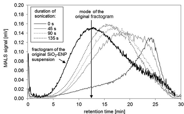
Fig. 3 Effect of increasing time of sonication after particle stabilisation in 0.025% FL-70™ and pH adjustment on AF<sup>4</sup> fractogram.
