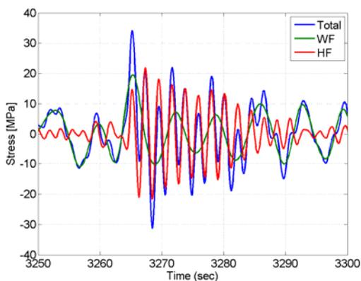
**Figure 5.** Stress measurements amidships on a large container vessel in a high sea-state. Direct wave-induced stresses on the rigid hull (WF), slamming-induced whipping stresses (HF) and the total combined stress [3]
