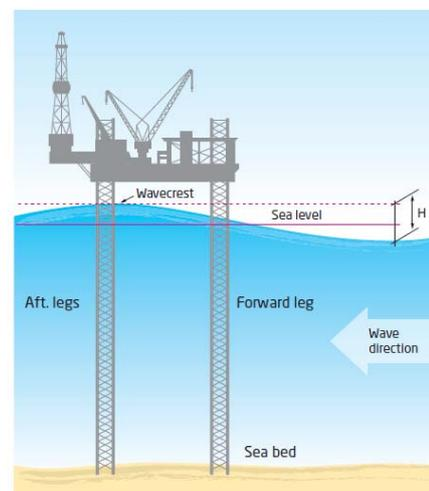
**Figure 9.** Overturning wave loading on a jack-up rig
