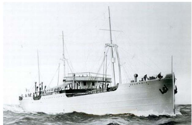
**Figure 1.** The *MS Selandia*, the first ocean-going diesel motor ship, carrying 6,800 DWT, built by B&W in 1912 and assigned to the EAC (<http://selandia100.dk/contact-2>)
