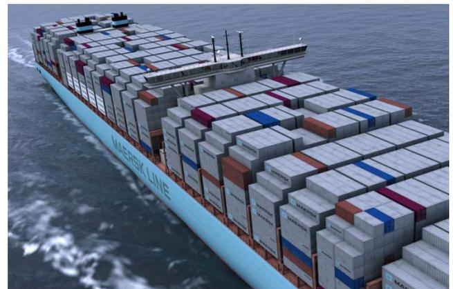
**Figure 3.** The *Triple E*, an example of the new generation of large containerships; it is 400 m long and 59 m wide, has a speed of 19 knots and carries 165,000 DWT
