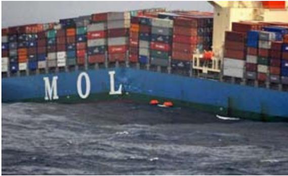
**Figure 4.** An example of a ship hull that was broken due to wave-induced stresses in the hull girder ([http://www.rina.org.uk/mol\\_comfort\\_accident.html](http://www.rina.org.uk/mol_comfort_accident.html))
