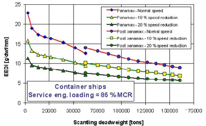
**Figure 2.** EEDI (energy-efficiency design index) in gCO<sub>2</sub> /ton\*mile as a function of size for different speeds [2]
