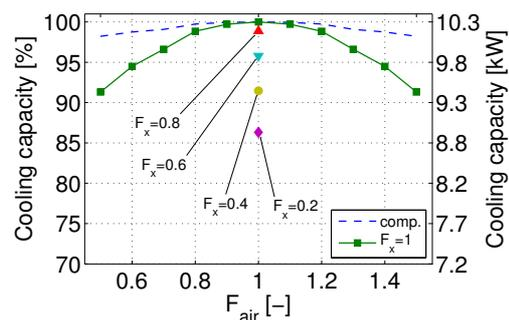
Figure 3: Evaporator capacity vs. individual maldistribution source.
