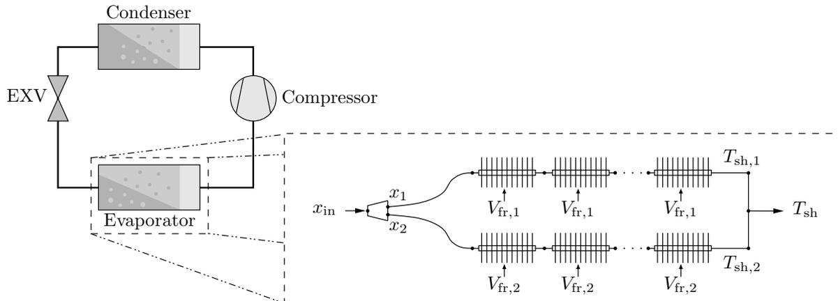
Figure 1: Sketch of the model setup
