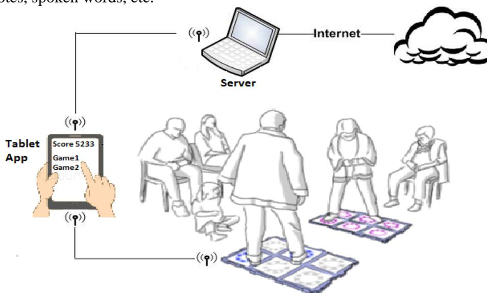
*Figure 1. The tablet app is developed to easily control games on modular tiles and to allow different kinds of feedback (e.g. score and sounds as immediate feedback, and collection of score on the internet, e.g. to document health effect from using the modular tiles).*
