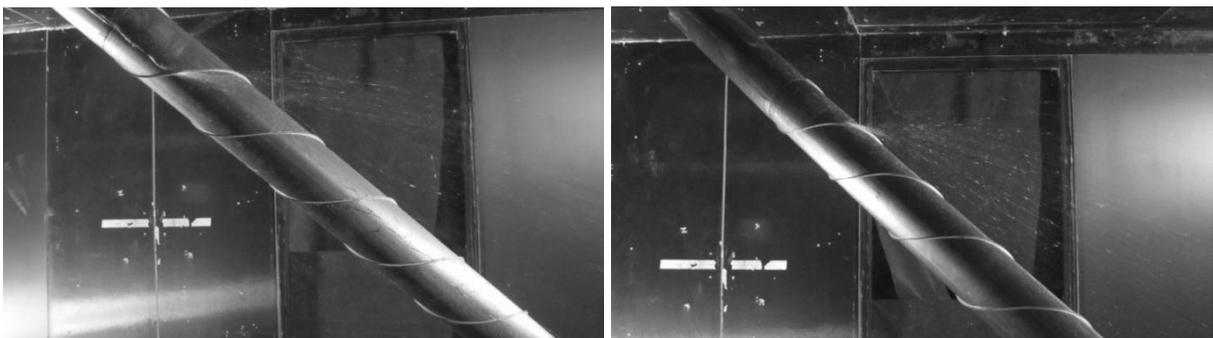
*Figure 9. Model F with helical strakes completely suppressing the rivulets. Lower rivulet at 14 m/s (left) and upper rivulet at 14 m/s (right).*
