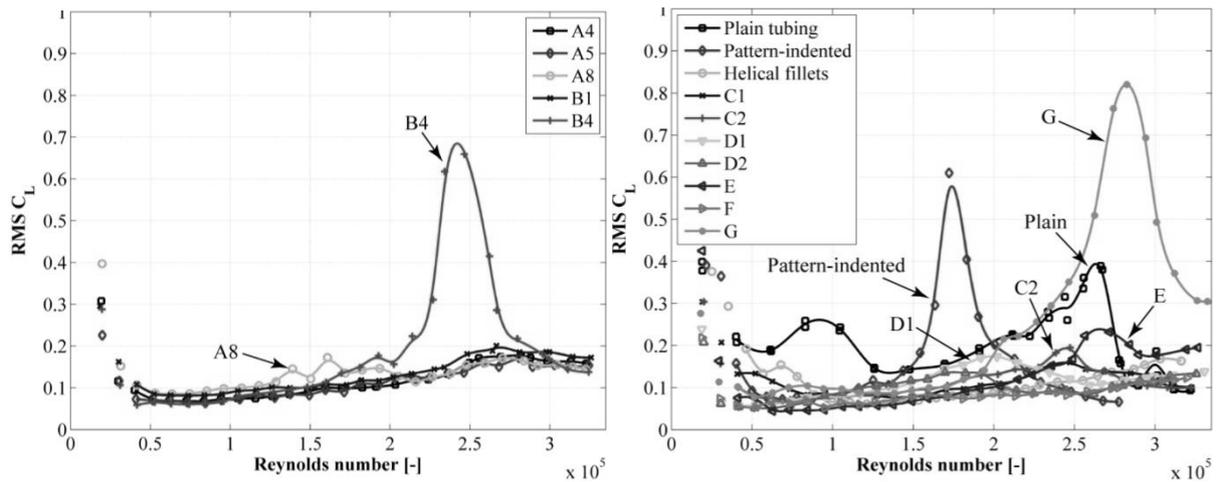
Figure 3. RMS values for the static lift force coefficients. Surface modified models with CVGs (left) and remaining surface modified models including currently applied cables (right).
