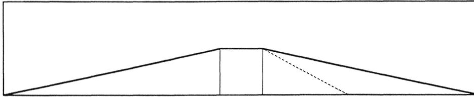
Figure 5: The two different “hills” considered in Approach 2. The thick line is the 1 : 5 slope in front and at the back, whereas the dashed line is the 1 : 2 slope at the back. The square box in the middle is the container seen from the side.
