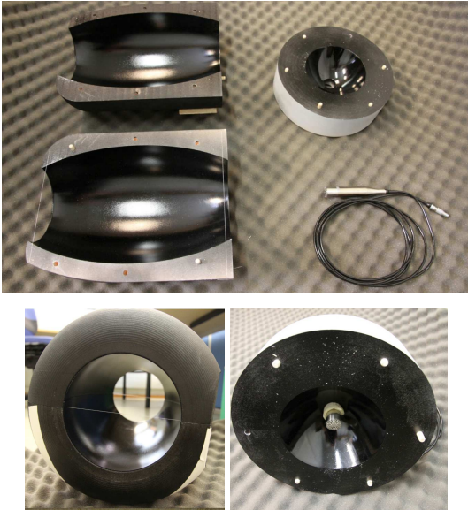
Fig. 3: Constructed reflectors. Up: all pieces separately. Down left: two sides together. Down right: the head piece and microphone together.
