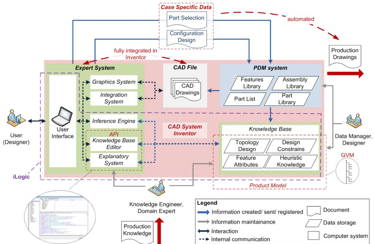
Figure 1 Integrated system architecture for automated precast design
