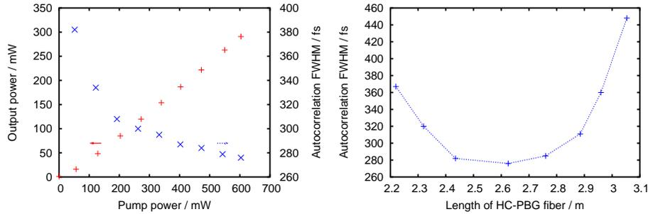
Fig. 4. Left: Output power and output autocorrelation FWHM (of the top envelope) after the HC-PBG fiber. Right: Cut-back of HC-PBG fiber at the highest pump power.
