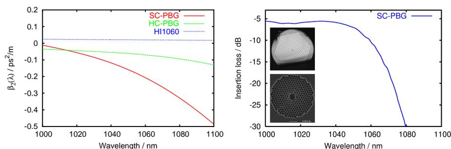
Fig. 1. Left: Dispersion of the SC-PBG, HC-PBG and standard fiber. Right: The insertion loss of the 0.36 m long SC-PBG fiber. The insertion loss is relative high compared to other components, but can be compensated by the high single pass gain of ytterbium. Insert: image of the SC-PBG fiber (top) and HC-PBG fiber (bottom).
