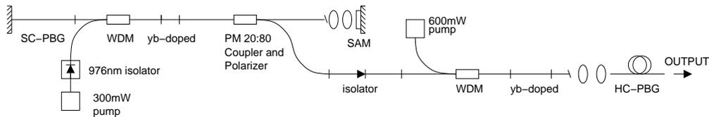
Fig. 2. Diagram of the laser system.
