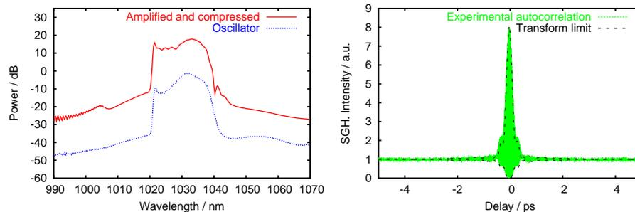
Fig. 3. Left: Output spectrum from the oscillator and output spectrum after the amplifier and compressor at maximum amplification. Right: Experimental autocorrelation trace at maximum amplification. The autocorrelation trace is compared to the autocorrelation trace of the transform limited pulse, and the deconvoluted pulse duration is 158 fs (FWHM).
