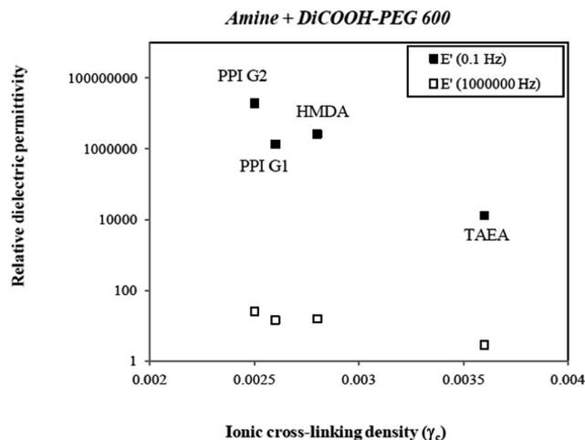
Fig. 6 Relative dielectric permittivities ( $\epsilon'$ ) at 0.1 and  $10^6$  Hz, respectively, of the ionic structures (four types of amines + DiCOOH-PEG 600) as a function of ionic cross-linking density.
