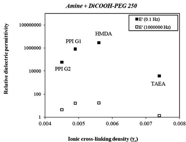
Fig. 5 Relative dielectric permittivities ( $\epsilon'$ ) at 0.1 and  $10^6$  Hz, respectively, of the ionic structures (four types of amines + DiCOOH-PEG 250) as a function of ionic cross-linking density.
