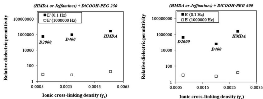
Fig. 7 Relative dielectric permittivities ( $\epsilon'$ ) at 0.1 and  $10^6$  Hz, respectively, of supramolecular ionic polymers from di-functional reactants as a function of ionic cross-linking density.
