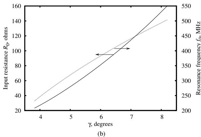
Fig. 9. Properties of the SSR antenna as a function of angle  $\gamma$ : (a) ratio  $Q/Q_{LB}$  and the relative radiated power of the  $TM_{11}$  mode; (b) input resistance at resonance and the resonance frequency.
