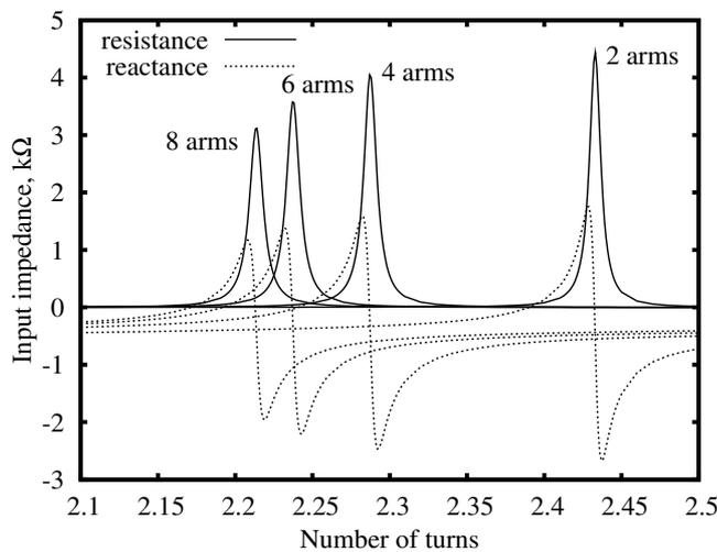
Fig. 3. Input impedance of the TE<sub>10</sub> MSH antenna as a function of the number of turns in each arm.
