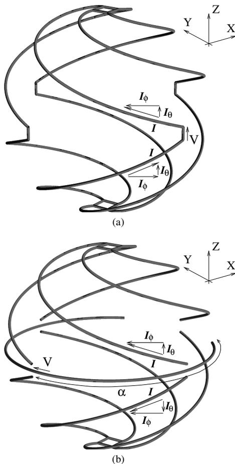
Fig. 2. Multiarm spherical helix (MSH) antenna: (a) TM<sub>10</sub> (electric dipole); (b) TE<sub>10</sub> (magnetic dipole).
