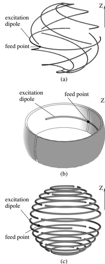
Fig. 1. Geometries of spherical magnetic dipole ( $TE_{10}$  mode) antennas: (a) Multiarm spherical helix (MSH) antenna; (b) spherical split-ring resonator (S-SRR) antenna; (c) spherical split ring (SSR) antenna.
