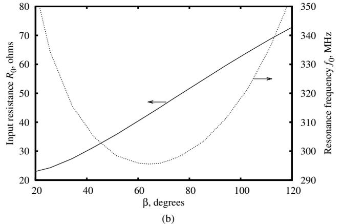
Fig. 6. Properties of the S-SRR antenna as a function of angle  $\beta$ : (a) ratio  $Q/Q_{\text{LB}}$  and the relative radiated power of the TM<sub>11</sub> mode; (b) input resistance at resonance and the resonance frequency.
