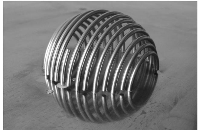
Fig. 11. Fabricated prototype the SSR antenna.
