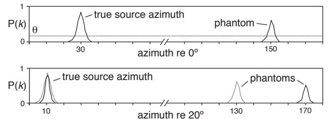
**Fig. 1.** Head movement strategy. Top: Two candidate azimuths are identified above the threshold  $\theta$ . Bottom: After head rotation by  $20^\circ$ , only the azimuth candidate at  $10^\circ$  agrees with the azimuth-shifted candidate from the first signal block (dotted line).
