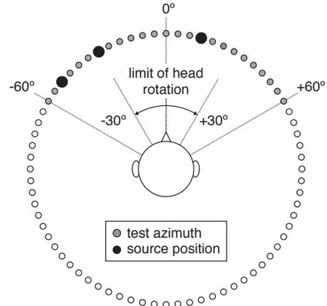
**Fig. 2.** Schematic diagram of the virtual listener configuration, showing azimuths used for testing (filled circles). Black circles indicate source azimuths in a typical three-talker mixture (in this example, at  $-50^\circ$ ,  $-30^\circ$  and  $15^\circ$ ). All azimuths were used for training. During testing, head movements were limited to the range  $[-30^\circ, 30^\circ]$ .
