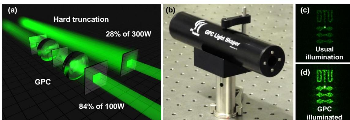
To obtain a uniformly illuminated rectangle with 84W, up to 216W is normally blocked. GPC, on the other hand can use 84W out of 100W, saving 200W (93%) (a). The compact GPC-LS is shown with an enclosure that prevents dust (b). Alternatively, a GPC-LS could increase the brightness by ~3x for the same input power as seen in the holographic reconstructions (c-d).
