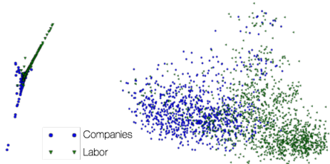
Figure 6. PCA on the 1st and 2nd principal components on the test dataset input vectors and output vectors from a 2000-500-250-125-10-DBN. Left: PCA on the 2000-dimensional input. Right: PCA on the 10-dimensional output.
