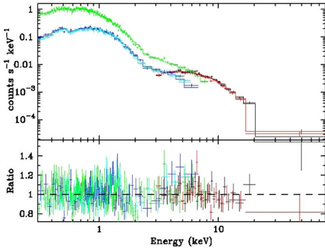
**Figure 5.** Count spectrum and model fit for our joint *XMM-Newton* and *NuSTAR* observation of Cen X-4, with the hard X-ray spectral cutoff included in the model. A bremsstrahlung model is shown:  $\text{tbabs}*(\text{nsatmos}+\text{bremss})$ . The color scheme is the same as in Figure 4. The fit parameters are shown in Table 1. (A color version of this figure is available in the online journal.)
