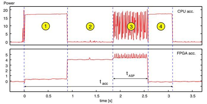
Fig. 4. Execution time in accelerator (1,000,000 calls).
