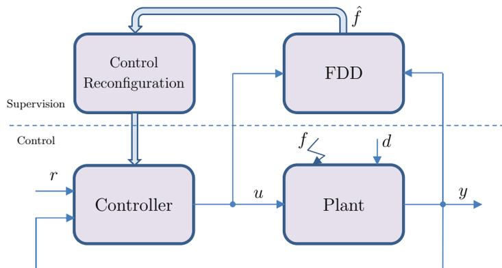
Figure 1: Structure of Active Fault Tolerant Control
