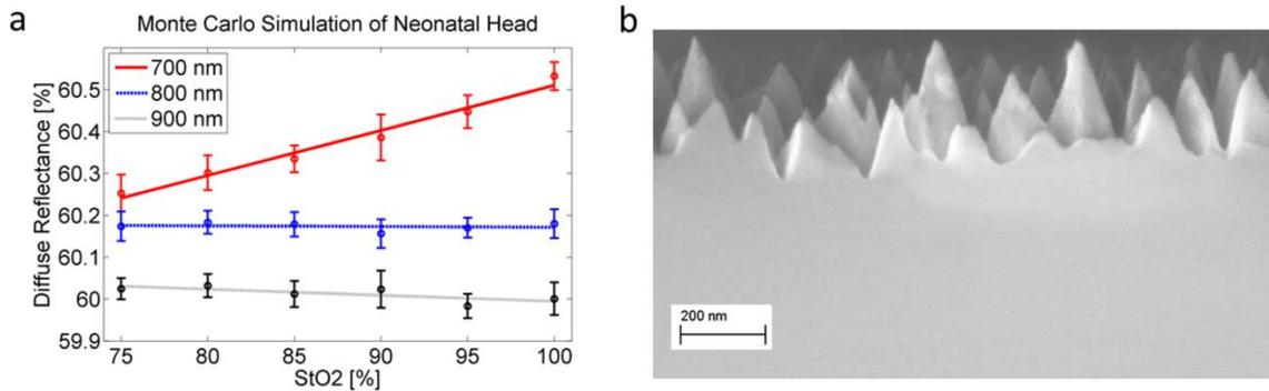
Fig. 2. (a) Results from Monte Carlo simulations. (b) SEM image of the black silicon nanostructures.
