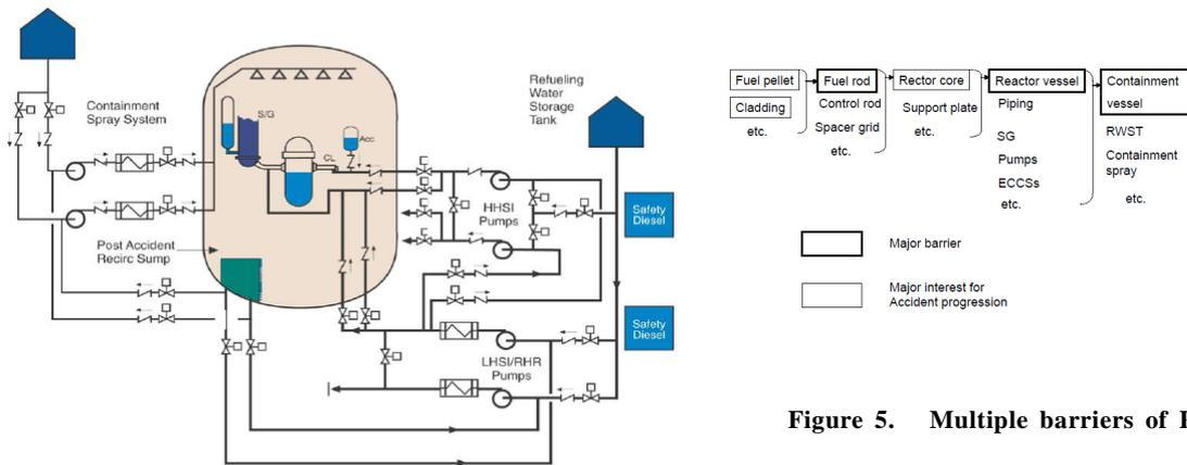
Figure 4. Safety system of conventional PWR plant
