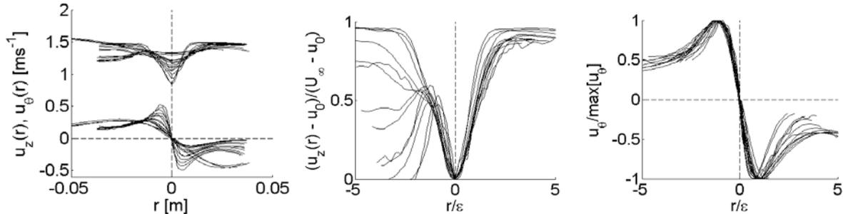
Figure 8: Velocity profiles from wind tunnel experiments for various angles and  $z/h = 2-13$ , showing the experimental values of the axial ( $u_z$ ) and azimuthal ( $u_\theta$ ) profiles (left column) and the axial (middle column) and azimuthal (right column) scaled by self-similarity variables.
