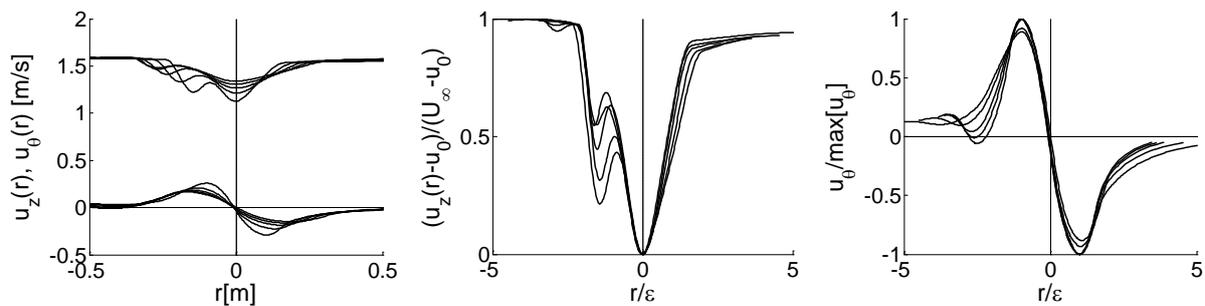
Figure 9: CFD velocity profiles at five plane positions  $z/h = 5-15$ . Left side shows the axial ( $u_z$ ) and azimuthal ( $u_\theta$ ) profiles and the middle and right sides show the axial and azimuthal profiles respectively, scaled by self-similarity variables.
