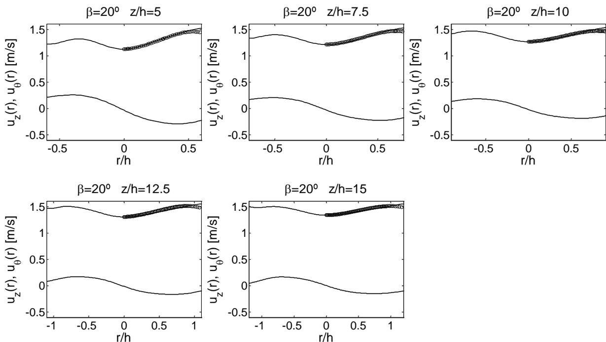
Figure 7: CFD velocity profiles of embedded vortices generated by a VG for a device angle  $\beta=20^\circ$ . Upper values are the axial velocity profile  $u_z$  and lower the azimuthal one  $u_\theta$ . CFD values of  $u_z$  are compared to the right-hand side of (4.1) calculated using the computational values  $u_\theta$  (o).
