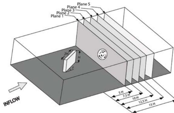
Figure 6: Plane location where the measurements were conducted.
