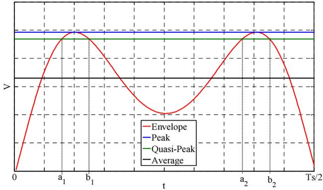
Fig. 8 Envelope, peak, quasi peak and average signals for the inductor current first harmonic across half line cycle
