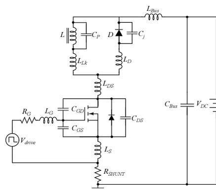
Fig. 1 DPT schematic with parasitic components
