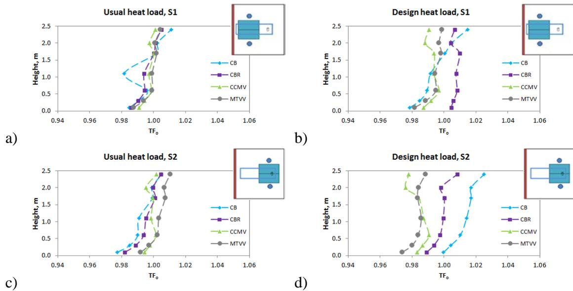
Figure 4. Averaged globe (operative) temperature factor (normalized globe (operative) temperature) in height for a) set-up 1 usual(low) heat load, b) set-up 1 design(high) heat load, c) set-up 2 usual(low) heat load and d) set-up 2 design(high) heat load.
