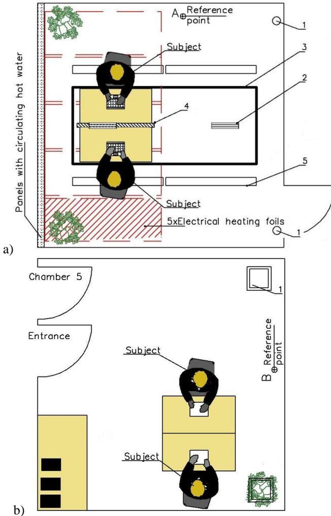
Fig. 1 Experimental set-up: a) exposure chamber; b) acclimatisation chamber.
