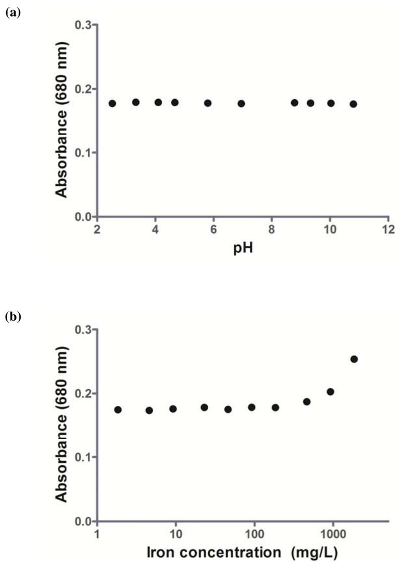
**Figure S3.** Effect of pH and residual iron ions concentration on phenol determination (added phenol concentration = 20  $\mu$ M)
