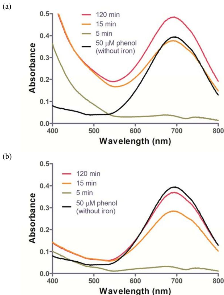
**Fig. 4. Spectra change by sample pretreatment using  $\text{Na}_2\text{CO}_3$  (Reagent C) (a) without (b) with addition of  $\text{Na}_2\text{CO}_3$ .**
