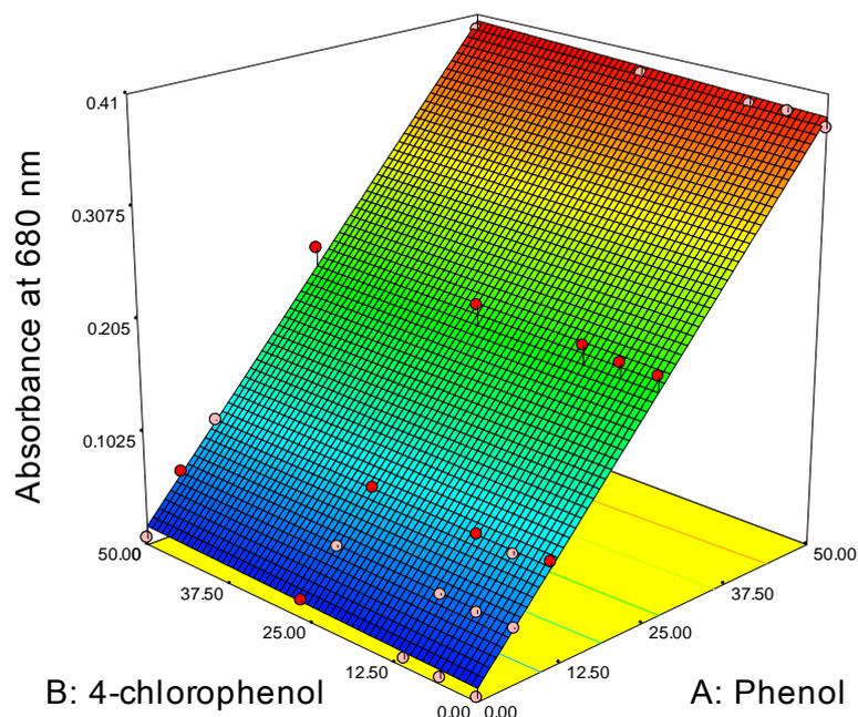
**Figure S1.** Response surface of absorbance at 680 nm for mixture of phenol and 4-chlorophenol after reaction with  $\text{NH}_2\text{Cl}$ .
