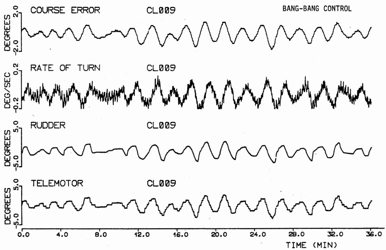
Fig. 16 Recordings from a test trial with Analog Steering gear of type 4 (RUN: CL008) and a Bang-Bang system of type 2 (RUN: CL009). Container ship with displacement 30.000 m<sup>3</sup> at 18.8 knots. The weather is calm, seastate 1. RUN: CL009 follows immediately after the end of RUN: CL008.
