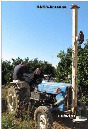
FIGURE 1 The tractor and the sensors used for data collection
