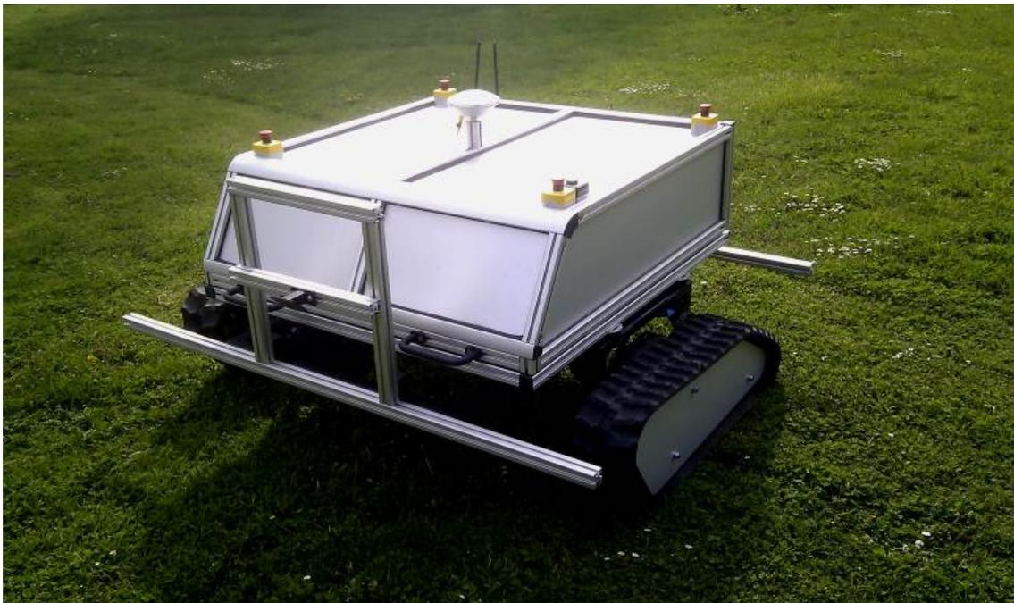
FIGURE 1: The electric powered belt driven platform (7 kW)
