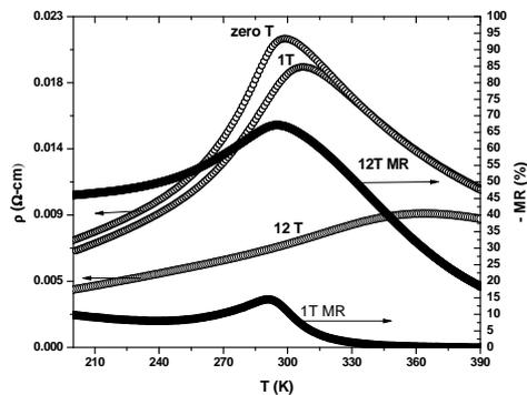
**Figure 3.** Temperature dependent electrical resistivity with right axis giving the percentage of magnetoresistance in 1T and 12T
