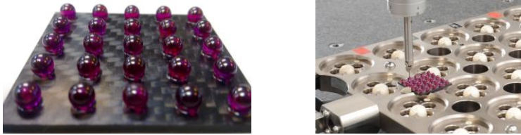
Figure 1: CT ball plate (left) and a setup for traceability transfer using a ball plate as part of the calibration procedure of the CT ball plate using CMM (right).
