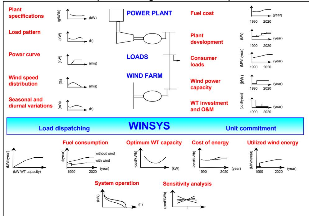
Figure 5 WINSYS: diagram showing input and output
