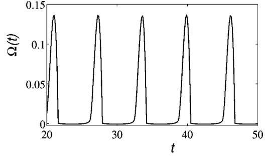
FIG. 3. Rotational velocity  $\Omega(t)$  (arbitrary units) in the case of dry friction with rational friction dependence  $\gamma(f) = \gamma_0(z_1 - f)/(f - z_2)$  and the driving force  $f(t) = f_0 \sin(\omega t)$ , computed numerically for  $\gamma_0 = 1$ ,  $z_1 = -z_2 = 1$ ,  $f_0 = 1/2$ , and  $\omega = 1$ .
