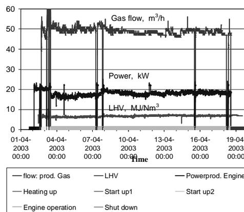
**Figure 3:** Plant performance during 400 hours experiment, April 2003.
