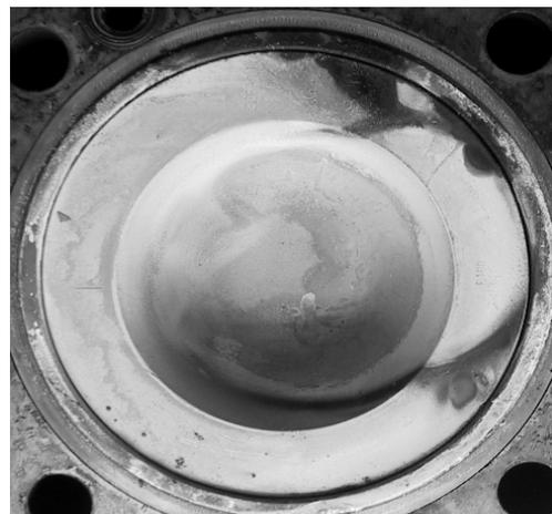
**Figure 5:** Top of cylinder after 1400 hours of operation.
