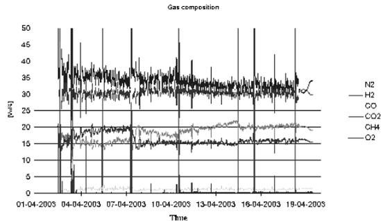
**Figure 4:** Gas composition during 400-hour experiment, April 2003.
